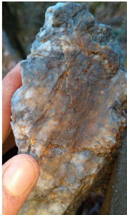
Figure 20. Quartz Reef with significant visible gold in the Victory United reef.
