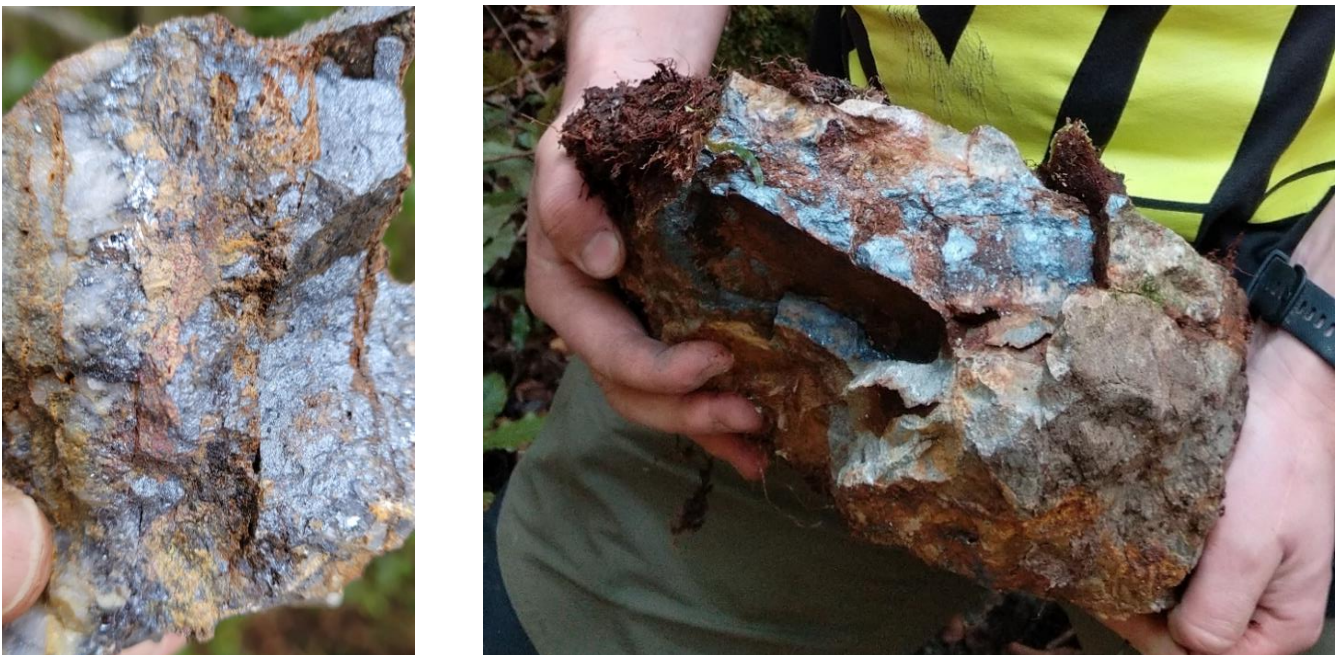
Figure 2. Massive stibnite veins at Auld Creek.
