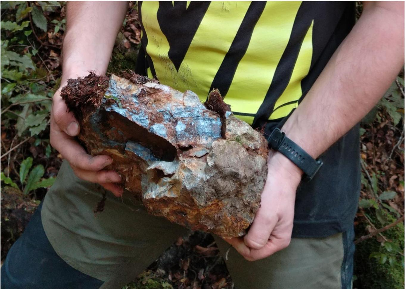
**Figure 3. Massive stibnite vein from the Fraternal Reef near FTTR001.**
